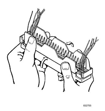
3.06 Snap latches on ends of sealant box to lock modules into place
