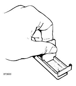
Note: When wire ports have been filled previously with sealant, it will be necessary to remove a small amount of grease from the new sealant box to allow easy module insertion. Use this procedure when ONE OR MORE of the modules in the rearrangement has previously been in a sealant box.
